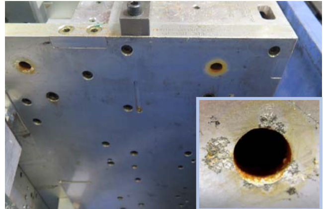
Image 2: Aluminum alloy mold with a close-up of deposits in the cooling channel and pitting.
