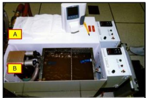
The side by side sumps were dosed with BCP™ 2430. The sump on the left (A) looks turbid, murky and gray, just after dosing. This is the typical appearance just after dosing BCP™ chemistry. In most cases, deposit removal is visually observable in minutes. The sump on the right (B) shows a structured foam or slurry; clearly, the “gunk” is in the process of being removed, and floated.
